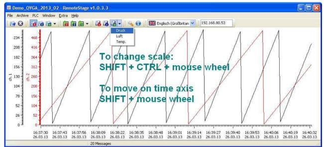
Above figure displays all archived trend with name "Druck" of the Panel-PLC / Panel-HMI with the IP-address 192.168.80.30. The time will be displayed in the Language format you assigned on your PC (here in German = DE)
