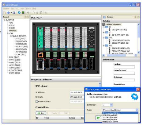
With the "ConfigStage" all external peripheries and intelligent drives compatible to CAN or Modbus RTU /TCP can be included into the S7-environment in an easy way without any knowledge about these communication technologies.
