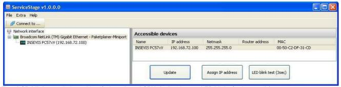
The "LCD-blink test" helps to identify the selected CPU. (yellow battery-LED blinks for 3 seconds).
